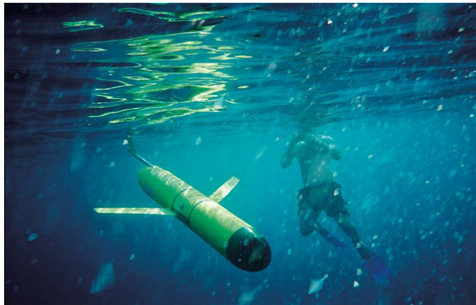
Figure 14: the Slocum G2 glider made by Teledyne Webb Research 16 .
