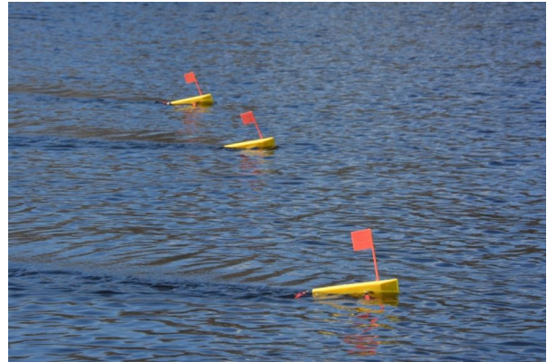
Figure 28: a) an example planar board used for trolling 30 and b) three planar boards in use during trolling operations 31 .
