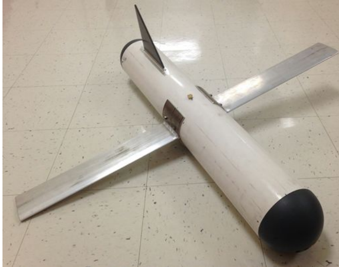
Figure 8: The SeaQPR 2.0, a glider design created by the Waver Rider team of academic year 2015.
