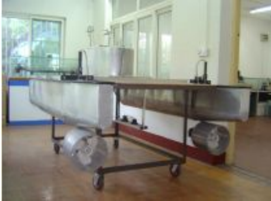
Figure 10: The two-hull design prototype including ducted propellers (left), and the ASV during testing (right)
